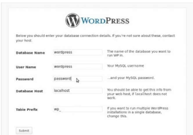
■ Adding the MySQL database settings during WordPress installation
