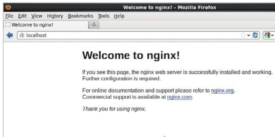
■ Testing that the Nginx installation has worked by pointing the browser at localhost
